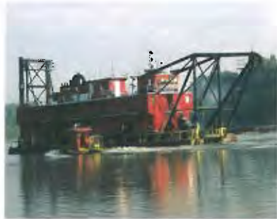
Dredge removing sediment from the Alabama River.
